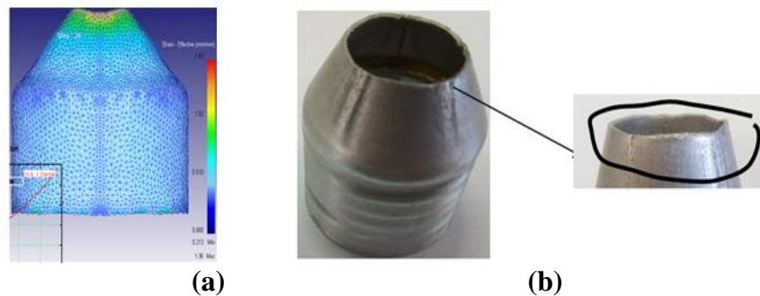
Fig. 23: Earing at conical semi-die angle 15^\circ , wall thickness 1mm and grease-lubricated. a) FE results and b) Experimental.
