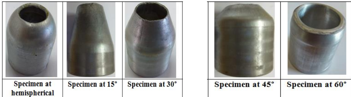
Fig.11 the deformed tubes after nosing process.
