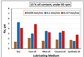
**Fig. 4** effect of oil type and feed rate on surface roughness of Al. under 95 rpm and 15 % oil content
