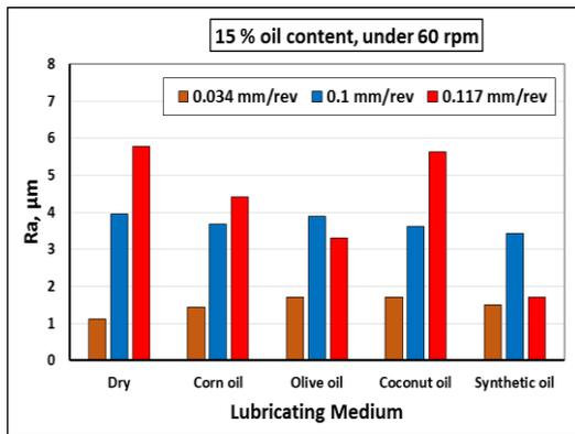
**Fig.1** effect of oil type and feed rate on surface roughness of Al. under 60 rpm and 15 % oil content
