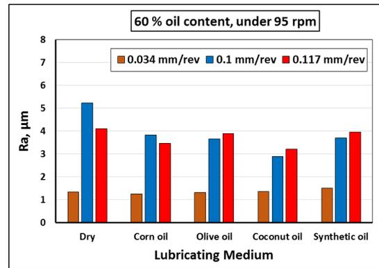
**Fig. 6** effect of oil type and feed rate on surface roughness of Al. under 95 rpm and 60 % oil content
