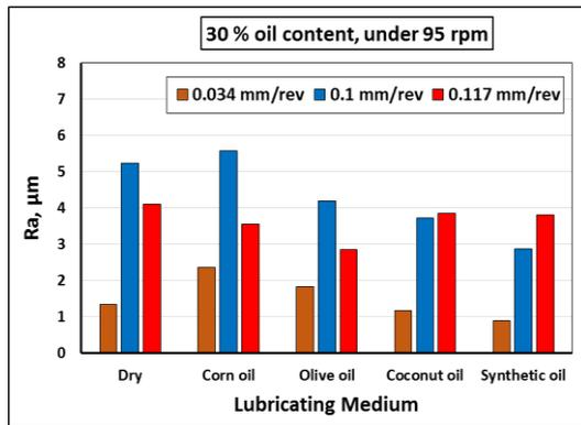
**Fig. 5** effect of oil type and feed rate on surface roughness of Al. under 95 rpm and 30 % oil content
