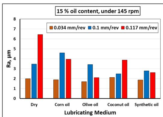
**Fig. 7** effect of oil type and feed rate on surface roughness of Al. under 145 rpm and 15 % oil content
