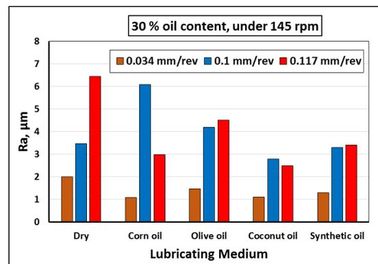
**Fig. 8** effect of oil type and feed rate on surface roughness of Al. under 145 rpm and 30 % oil
