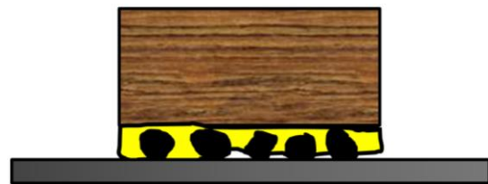
Fig. 10 Contact between relatively big rubber particles and ceramic surface.
