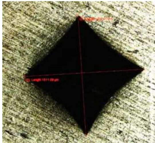
Fig. 2 The dimensions of the indenter on the counterface surface.
