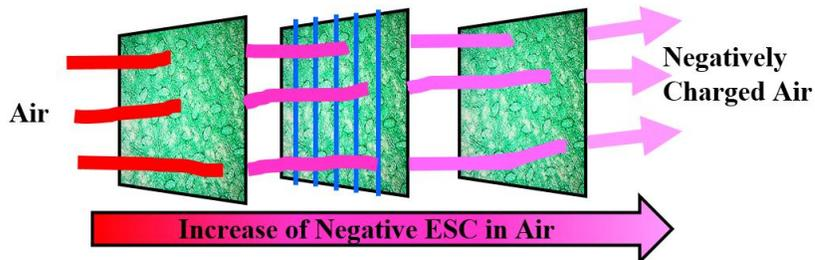
Fig. 5 Illustration of the increase of ESC generated on the surfaces of the PP layers.
