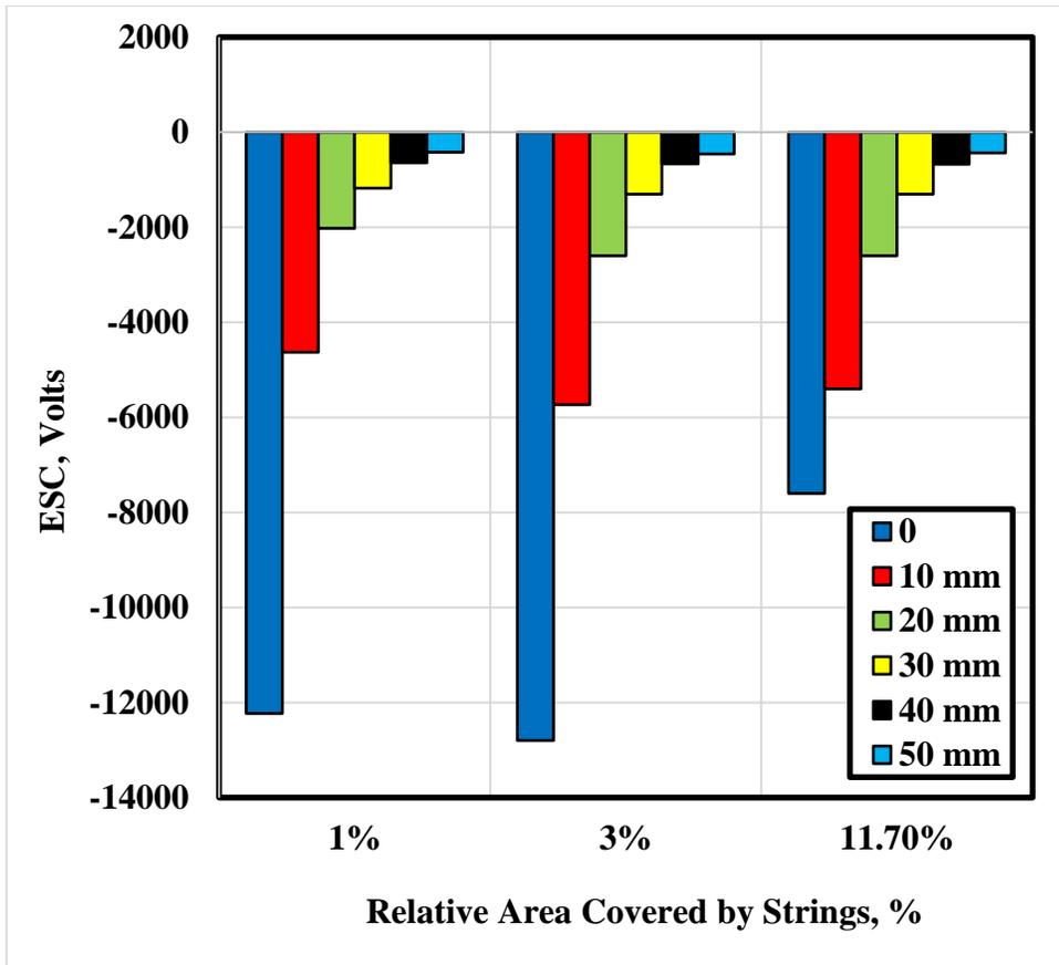
Fig. 10 Effect of the relative area covered by PET strings on ESC.
