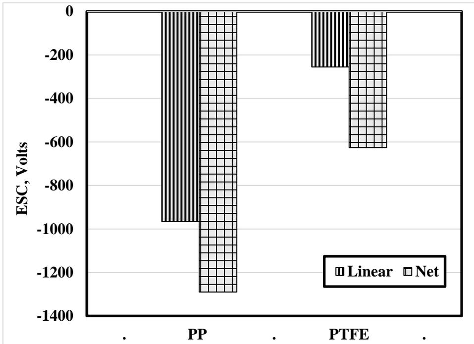
Fig. 8 ESC generated from PP separated by PP and PTFE strings.
