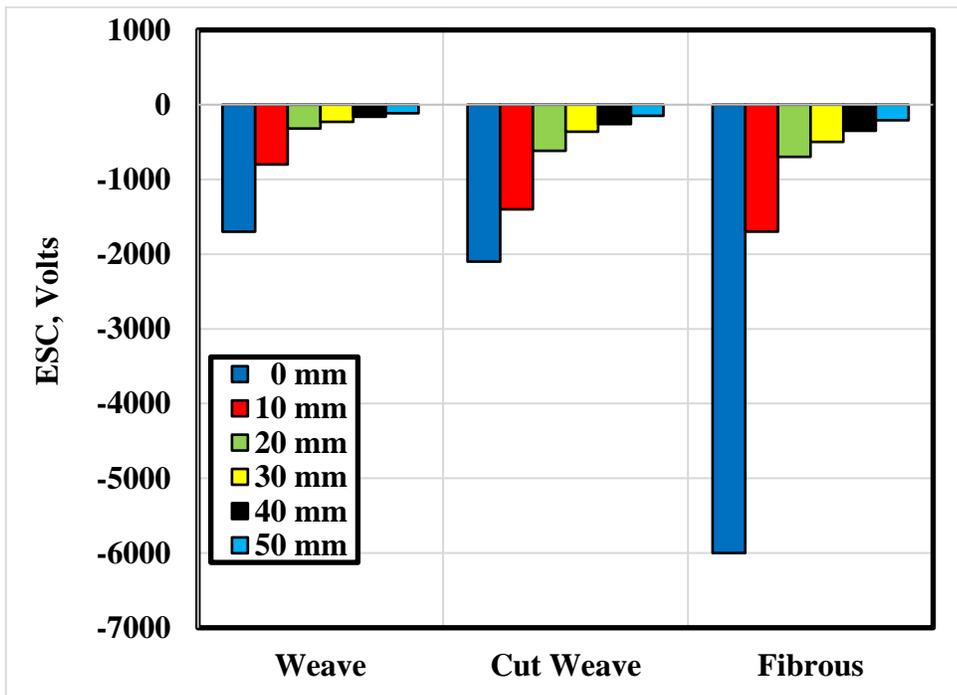
Fig. 11 Effect of the fibers of PET strings on ESC.
