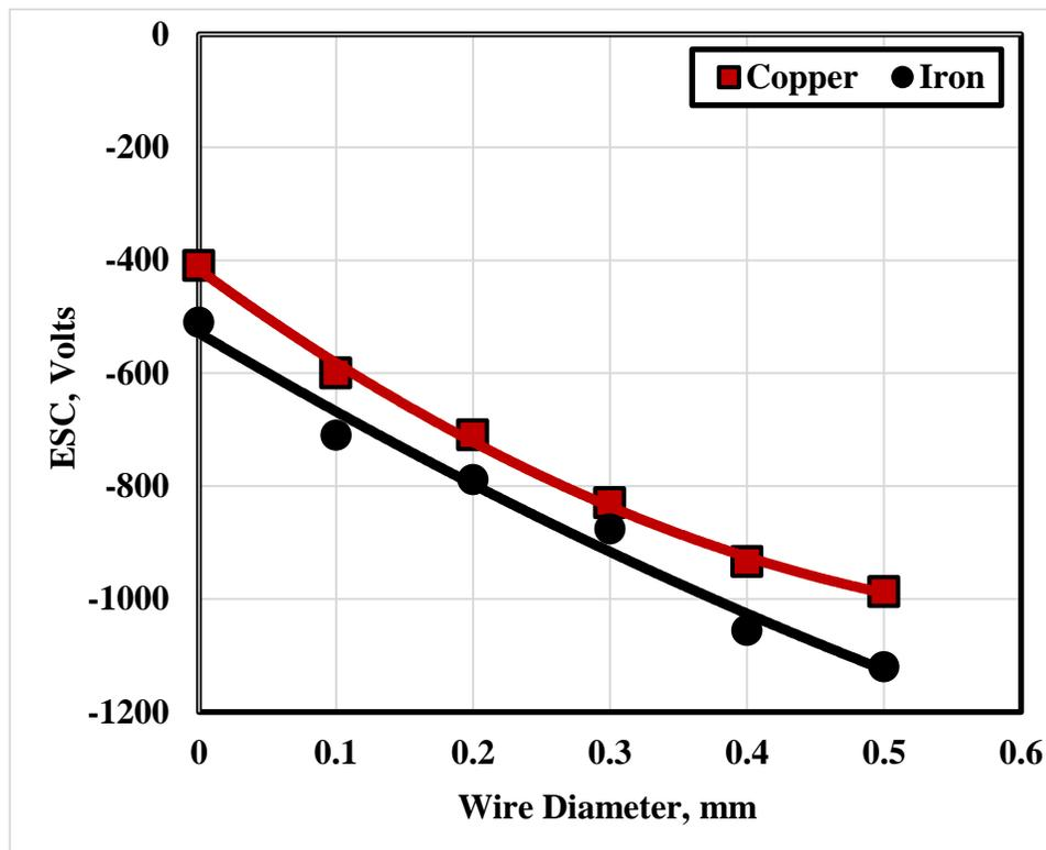
Fig. 5 ESC generated from PP separated by copper and iron wires of different diameters.
