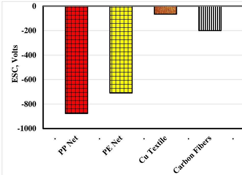
Fig. 7 ESC generated from PP separated by PP and PE net as well as copper textile and carbon fibers.
