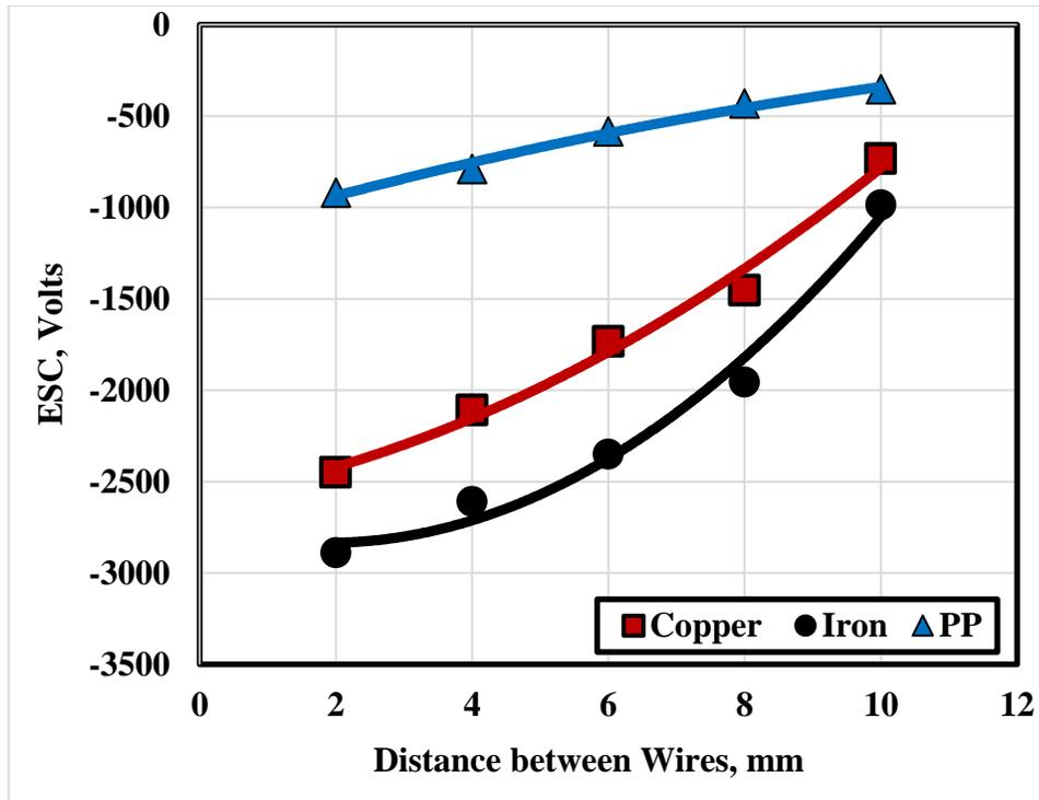
Fig. 4 ESC generated from PP separated by copper and iron wires as well as PP strings of 0.5 mm diameter.
