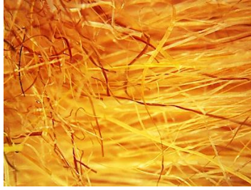
a. PET (I) Nonwoven of 0.02 mm fiber diameter.
