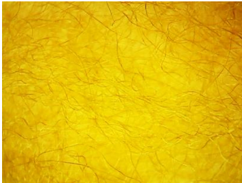
c. PET (II) Nonwoven of 0.01 mm fiber diameter.
