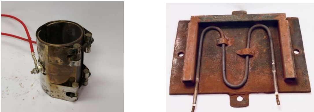
Fig. 2 Heaters for the compression and bending specimen's molds.
