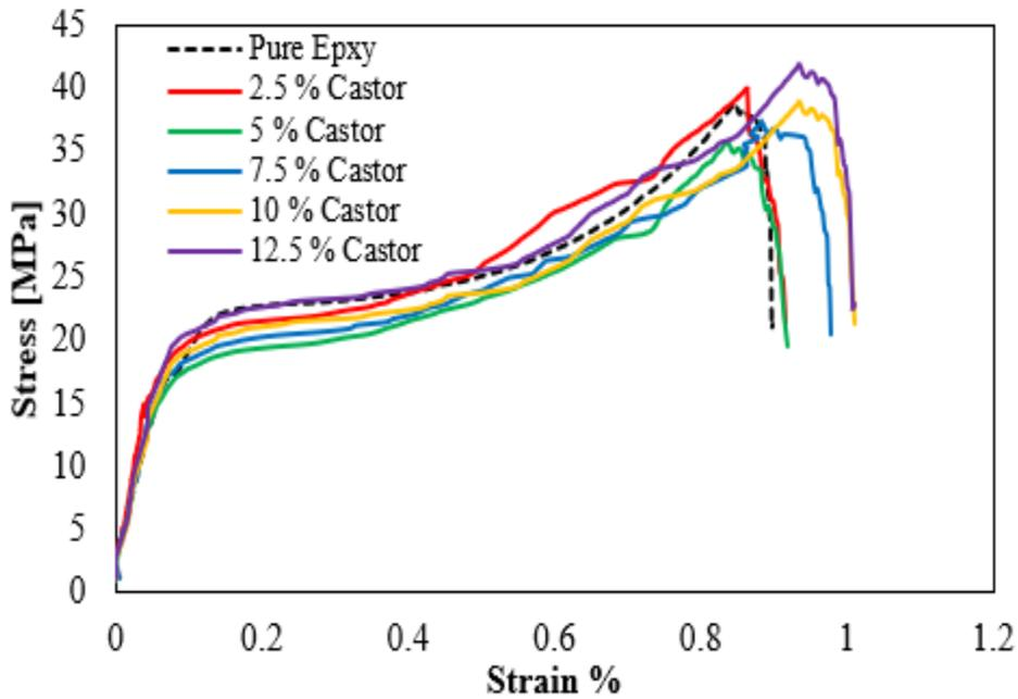
Fig. 3 Stress strain curve of epoxy resin filled with different filler content castor oil.
