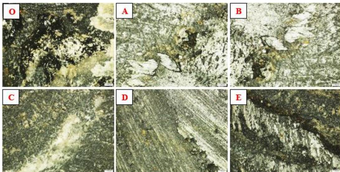
**Fig. 16** Optical topography images of epoxy matrix filled with palm oil, (O) free epoxy matrix, (A) 2.5 % palm oil, (B) 5 % palm oil, (C) 7.5 % palm oil, (D) 10% palm oil, and (E) 12.5 % palm oil.
