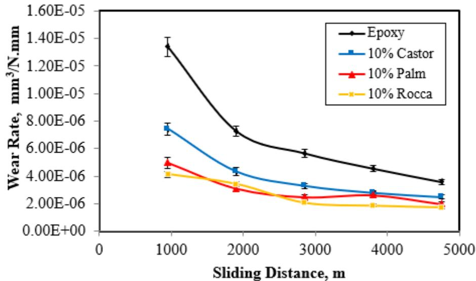
Fig. 14 Comparison of Wear rate between epoxy resin filled with different oils.
