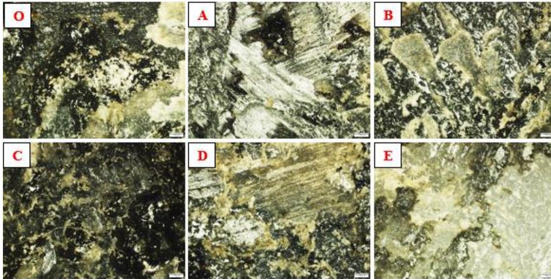
**Fig. 15** Optical topography images of epoxy matrix filled with castor oil, (O) free epoxy matrix, (A) 2.5 % castor oil, (B) 5 % castor oil, (C) 7.5 % castor oil, (D) 10 % castor oil, and (E) 12.5 % castor oil.
