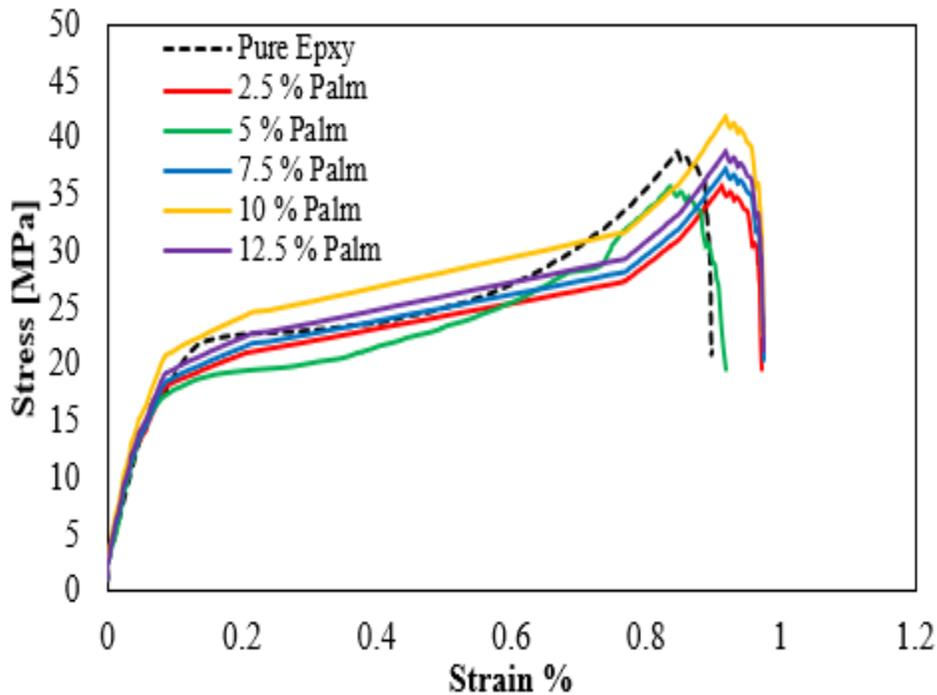
Fig. 4 Stress strain curve of epoxy resin filled with different filler content palm oil.
