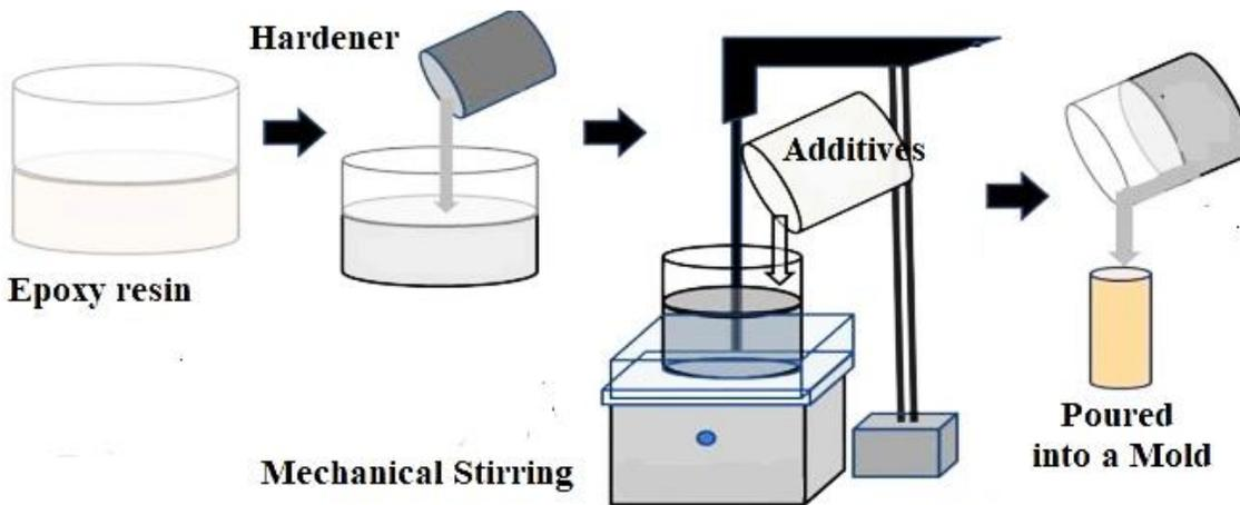
Fig. 1 Schematic diagram of epoxy sample preparation.
