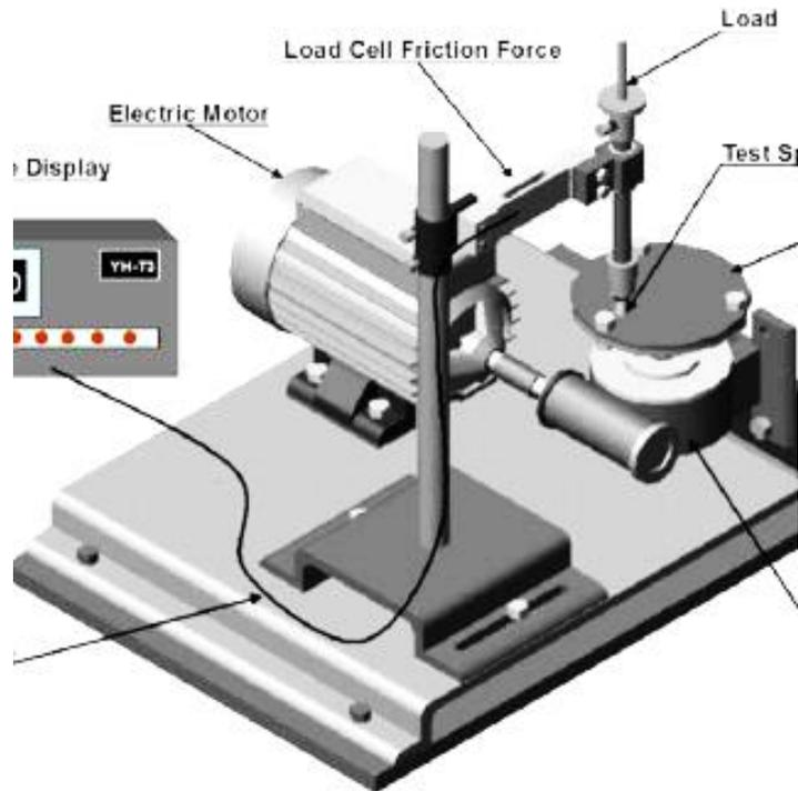
Fig. 2 Arrangement of tribometer test rig.
