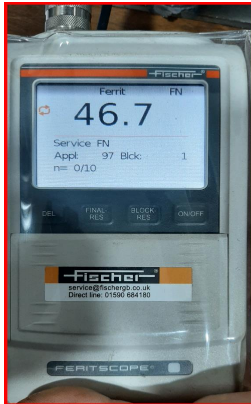
Fig. 5 Ferrite percentage content during measurement by using a ferrite-scope.
