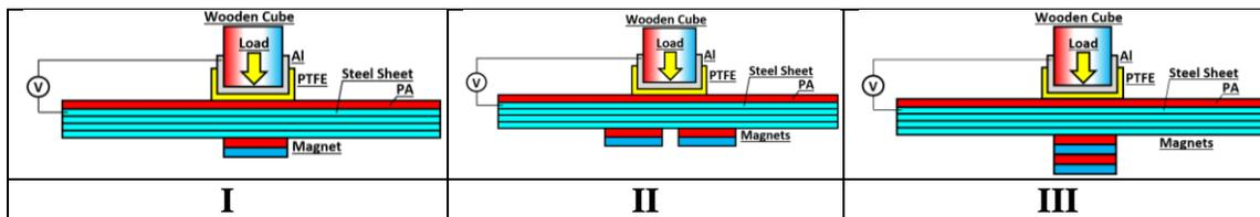
Fig. 3 Arrangements of the permanent magnets for steel sheets.
