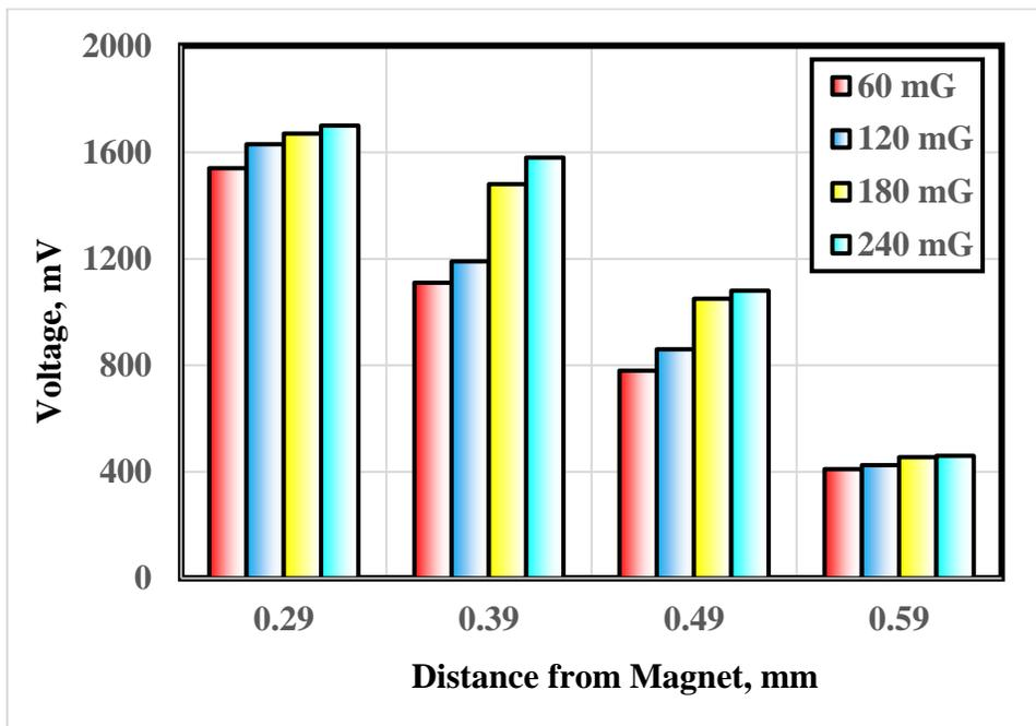
**Fig. 7 Voltage difference between PTFE and PA after sliding as function of the distance from the permanent magnets of the first group.**
