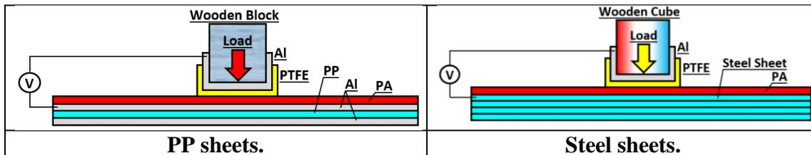
Fig. 1 Arrangement of the test procedure.
