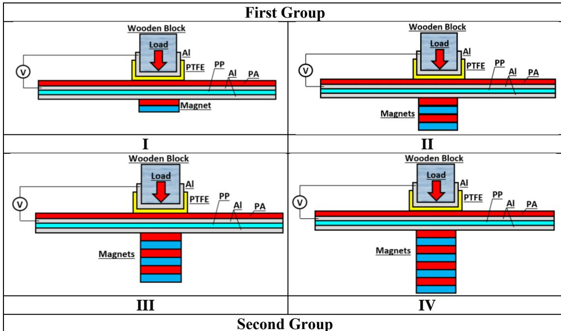
Fig. 2 Arrangements of the permanent magnets for PP sheets.
