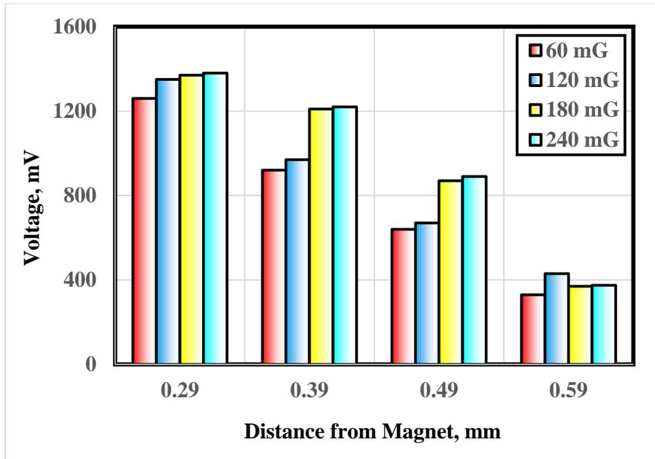
Fig. 5 Voltage difference between PTFE and PA after contact-separation as function of the distance from the permanent magnets of the first group.
