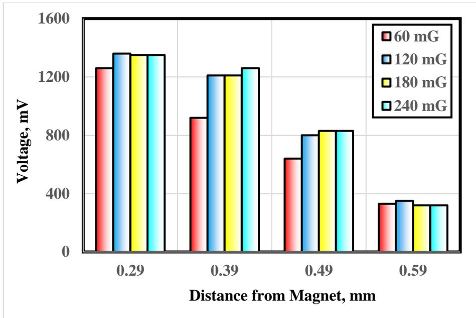
**Fig. 6 Voltage difference between PTFE and PA after contact-separation as function of the distance from the permanent magnets of the second group.**
