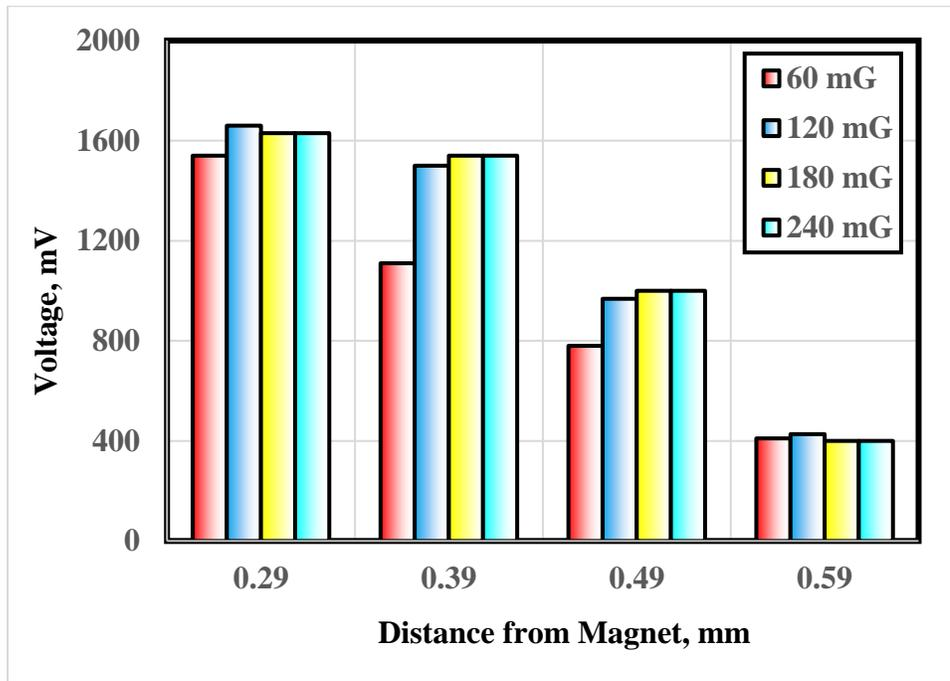
**Fig. 8 Voltage difference between PTFE and PA after sliding as function of the distance from the permanent magnets of the second group.**
