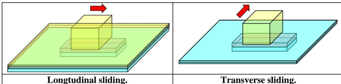
Fig. 4 Direction of sliding relative to the direction of the lines of magnetic field, [1].
