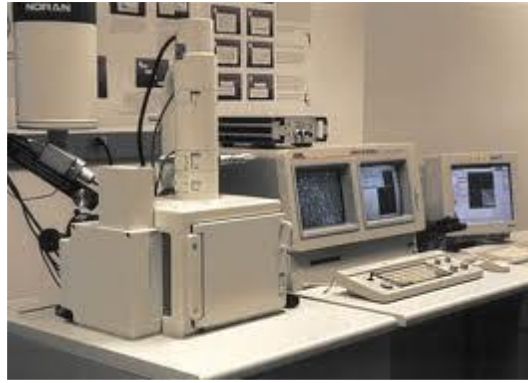
Fig. 5 Scanning Electron Microscopy JEOL-JSM 5400LV (30kv) with EDX and WDX400.
