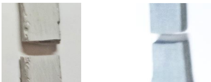
Fig. 7 fracture of both (a) Pure Epoxy (b) Epoxy with 0.2 wt. % MWCNTs.
