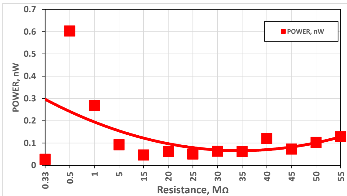
Fig. 14 Effect of external resistance on the power output of the Kapton button.
