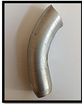
Figure. 7 The specimen after ECAP.
