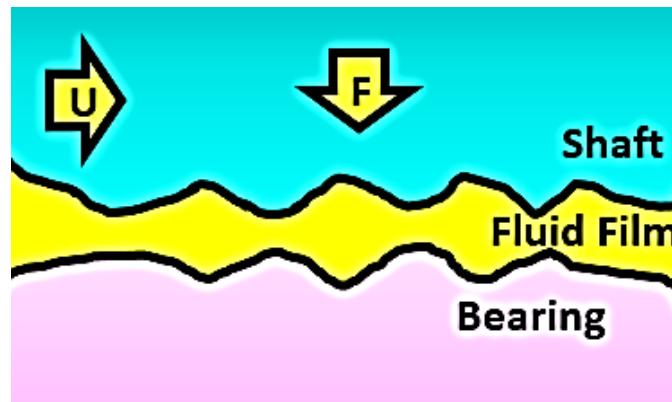
Fig. 5 Surface interaction at hydrodynamic lubrication regime.
