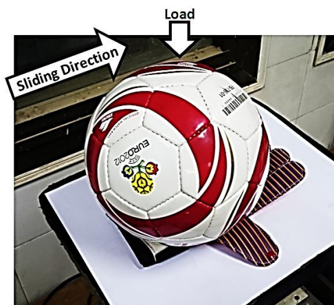
Fig. 1 Measurement of friction force between the ball and the glove.
