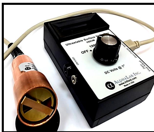
Fig. 1 Electrostatic field measuring device.
