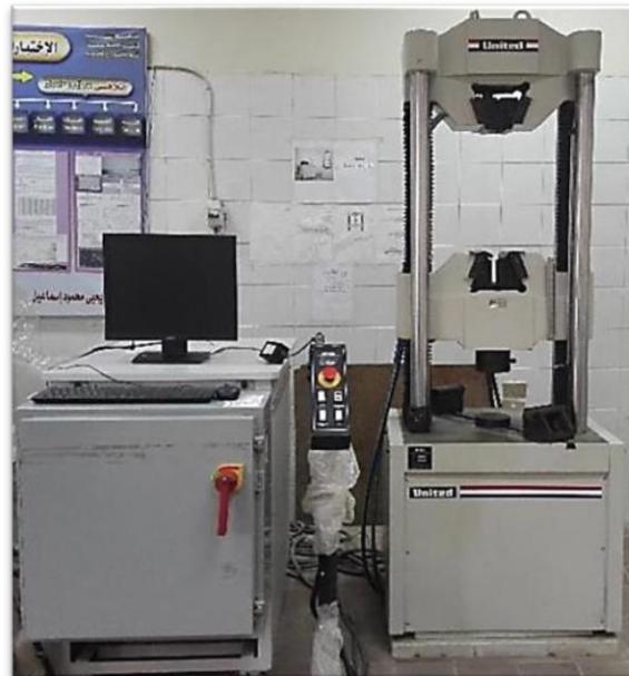
Fig. 8 Universal Testing Machine for compression test.
