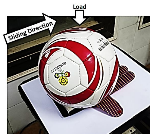
Fig. 2 Measurement of friction force between the ball and the glove.
