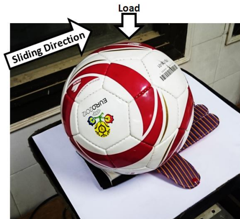
Fig. 1 Measurement of ESC generated from the sliding of the football against the glove.
