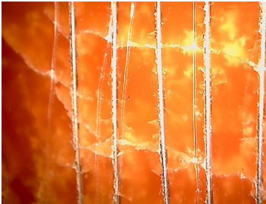
Fig. 3 Test specimen after scratch.
