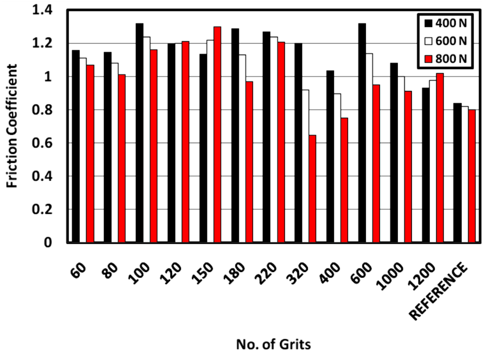
Fig. 5 Friction coefficient displayed by sport shoe sliding against dry emery paper of different number of grits.
