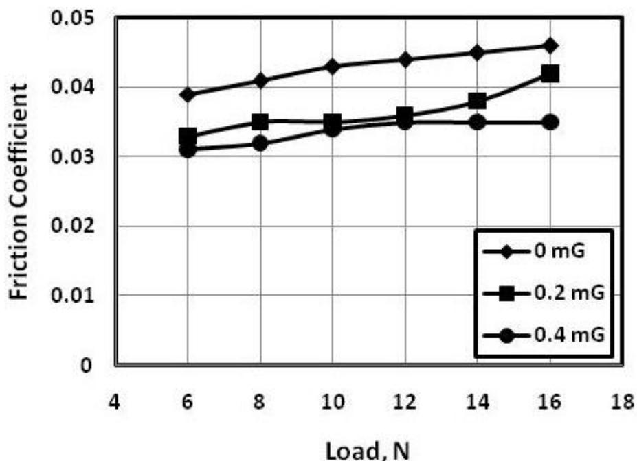
Fig. 7 Friction coefficient displayed by the sliding of steel pin against aluminium disc lubricated by oil dispersed by graphite.
