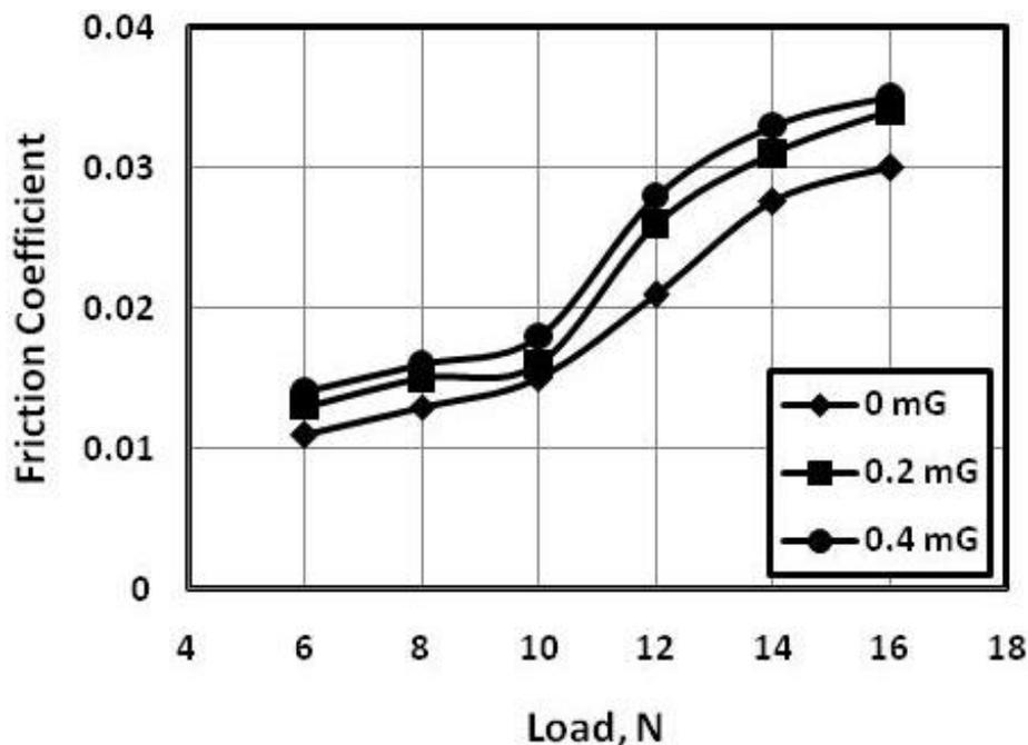
**Fig. 8 Friction coefficient displayed by the sliding of steel pin against aluminium disc lubricated by oil dispersed by DA.**
