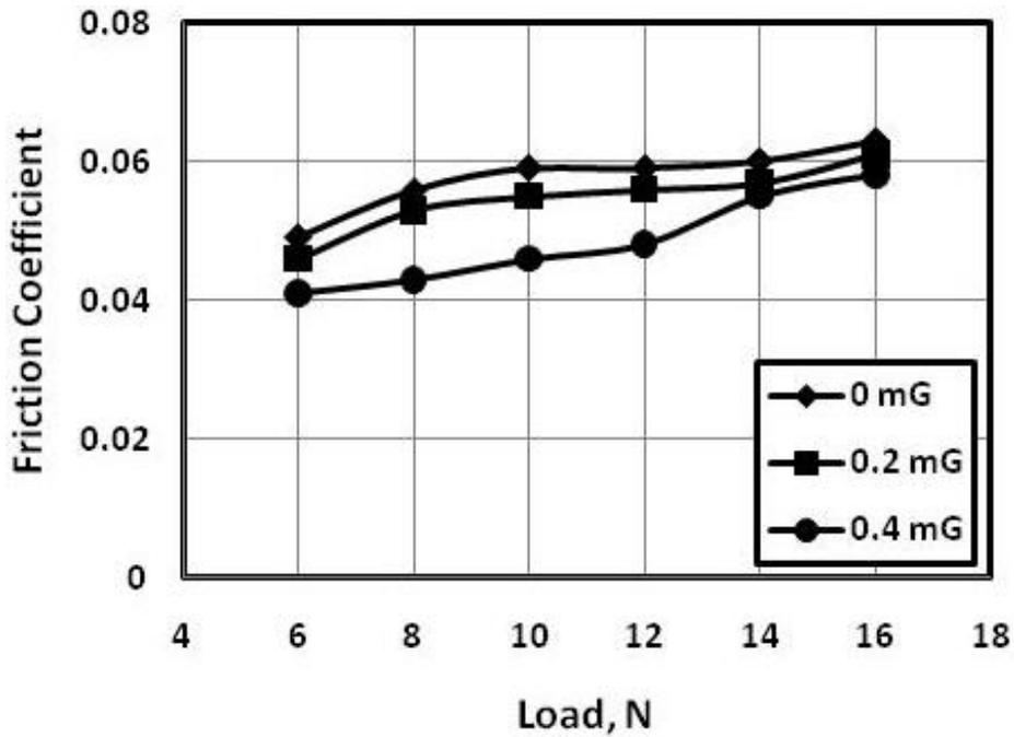
**Fig. 10** Friction coefficient displayed by the sliding of steel pin against aluminium disc lubricated by oil dispersed by PMMA.
