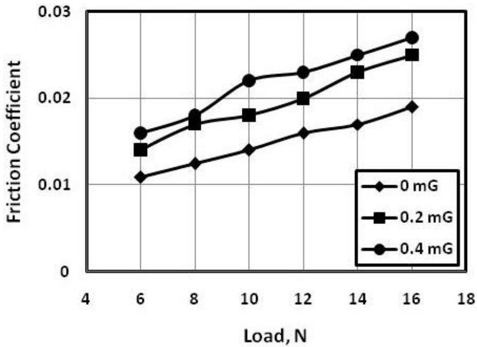
**Fig. 9** Friction coefficient displayed by the sliding of steel pin against aluminium disc lubricated by oil dispersed by PTFE.
