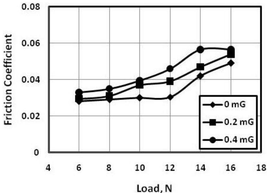
Fig. 4 Friction coefficient displayed by the sliding of steel pin against aluminium disc lubricated by oil dispersed by ZDDP.
