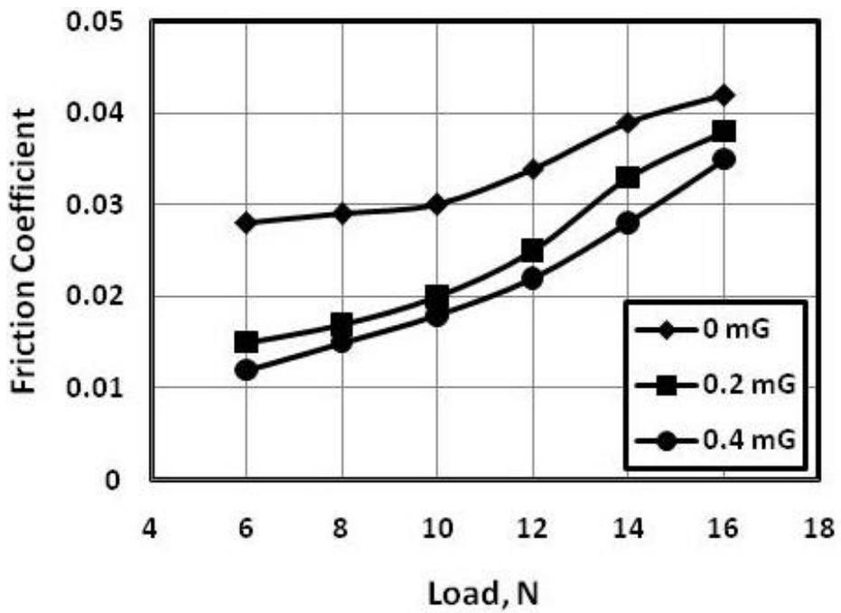
Fig. 6 Friction coefficient displayed by the sliding of steel pin against aluminium disc lubricated by oil dispersed by CMOC.
