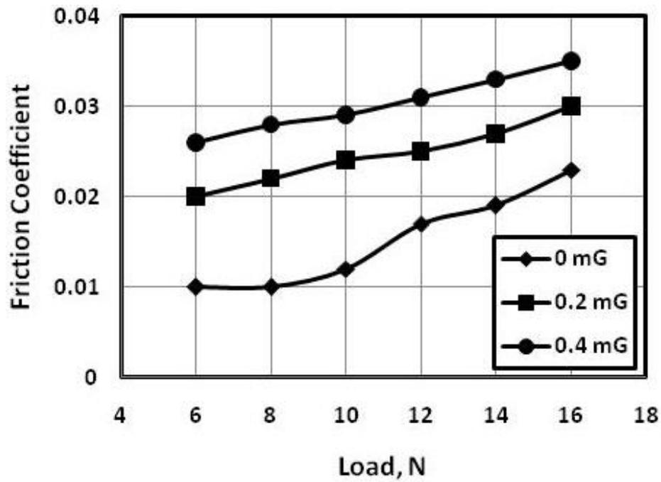
Fig. 5 Friction coefficient displayed by the sliding of steel pin against aluminium disc lubricated by oil dispersed by MoS<sub>2</sub>.
