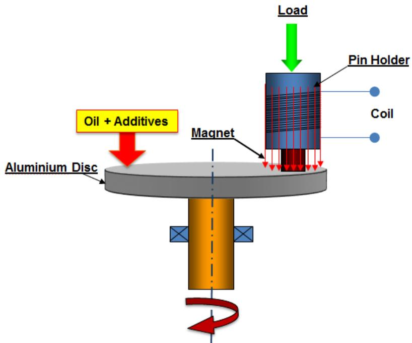
Fig. 2 Application of the magnetic field.
