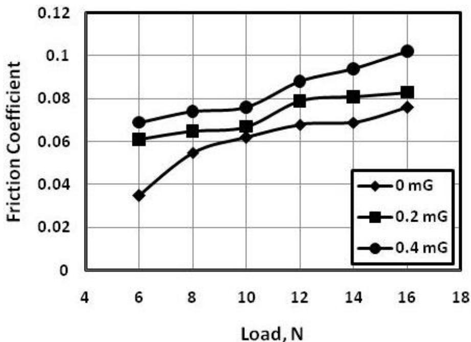
Fig. 3 Friction coefficient displayed by the sliding of steel pin against oil lubricated aluminium disc.
