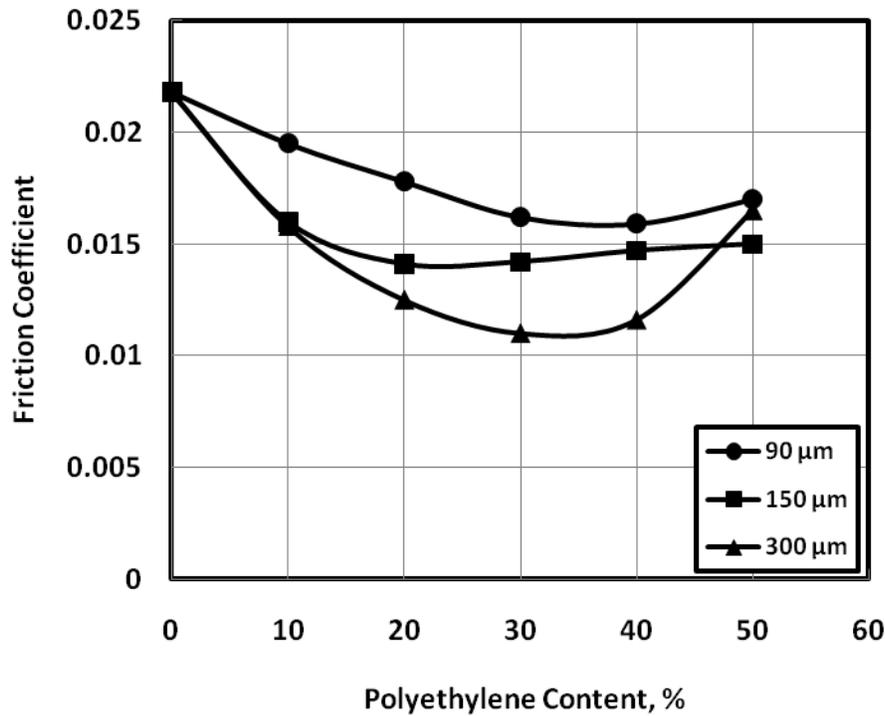
**Fig. 4 The effect of particle size of polyethylene dispersing grease on friction coefficient displayed by the test specimens.**
