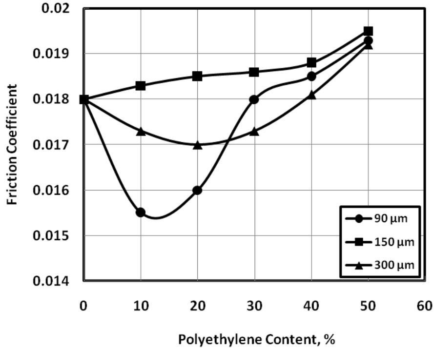
**Fig. 6** The effect of particle size of polyethylene dispersing abrasive contaminated grease on friction coefficient displayed by the test specimens.
