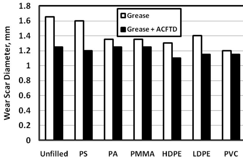
**Fig. 2 The effect of dispersing grease by polymeric powder and contaminating by sand particles on wear of test specimens.**
