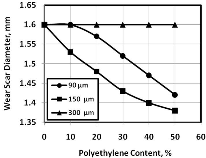
**Fig. 5** The effect of particle size of polyethylene dispersing grease on wear of the test specimens.
