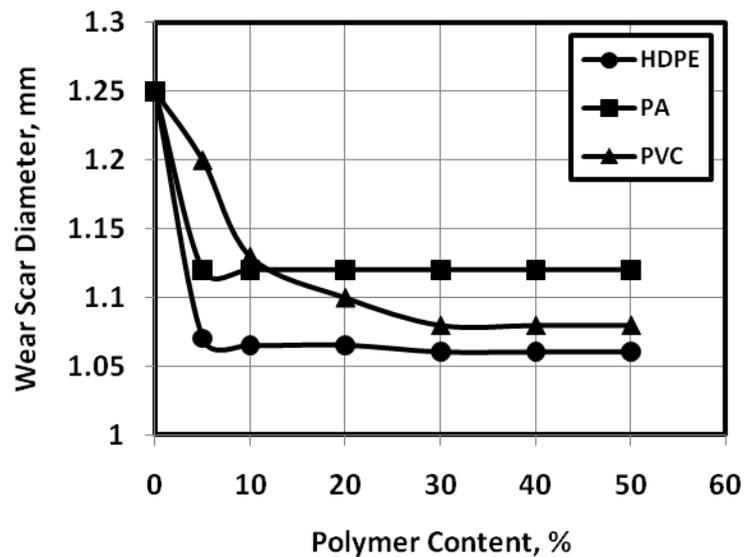
**Fig. 3** The effect of dispersing grease by polymeric powder on wear of test specimens.
