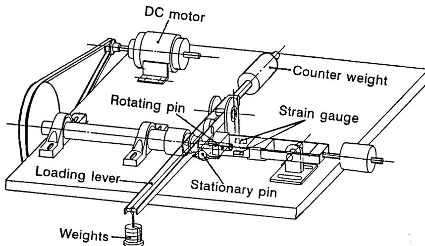
**Fig. 1** Arrangement of wear tester.
