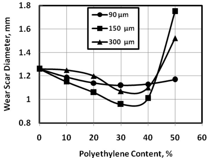
**Fig. 7 The effect of particle size of polyethylene dispersing abrasive contaminated grease on wear of the test specimens.**
