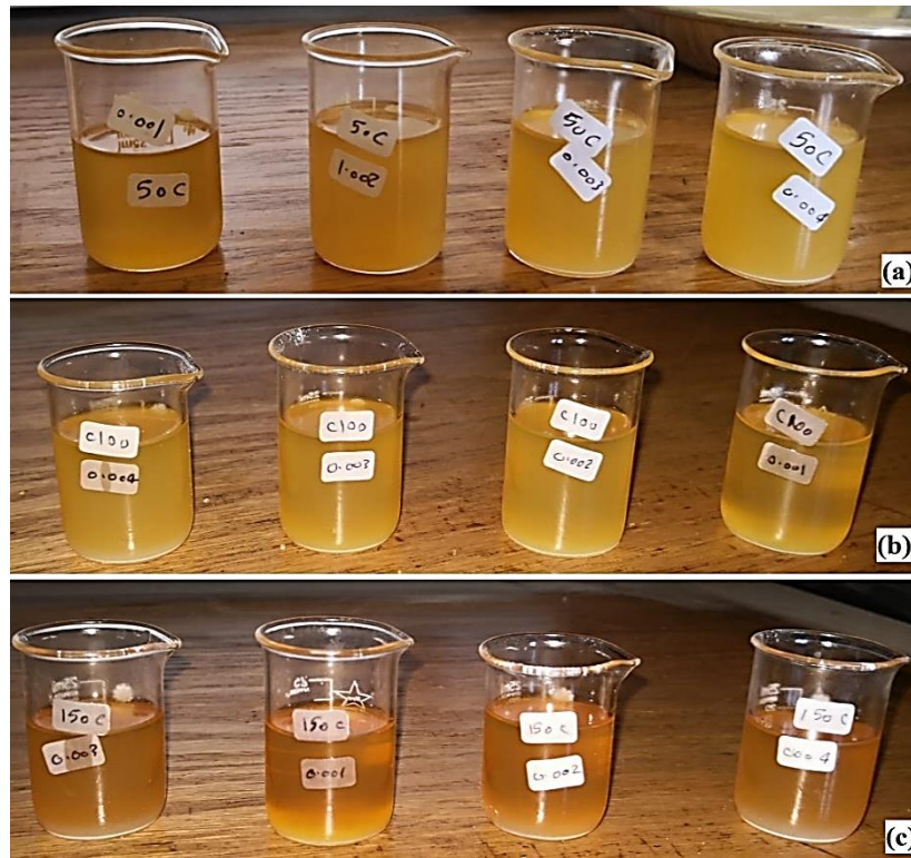
Fig. 3 Photograph of nano-lubricant oils carried out under mixing temperature (a) 50°C, (b) 100°C and (c) 150°C.
